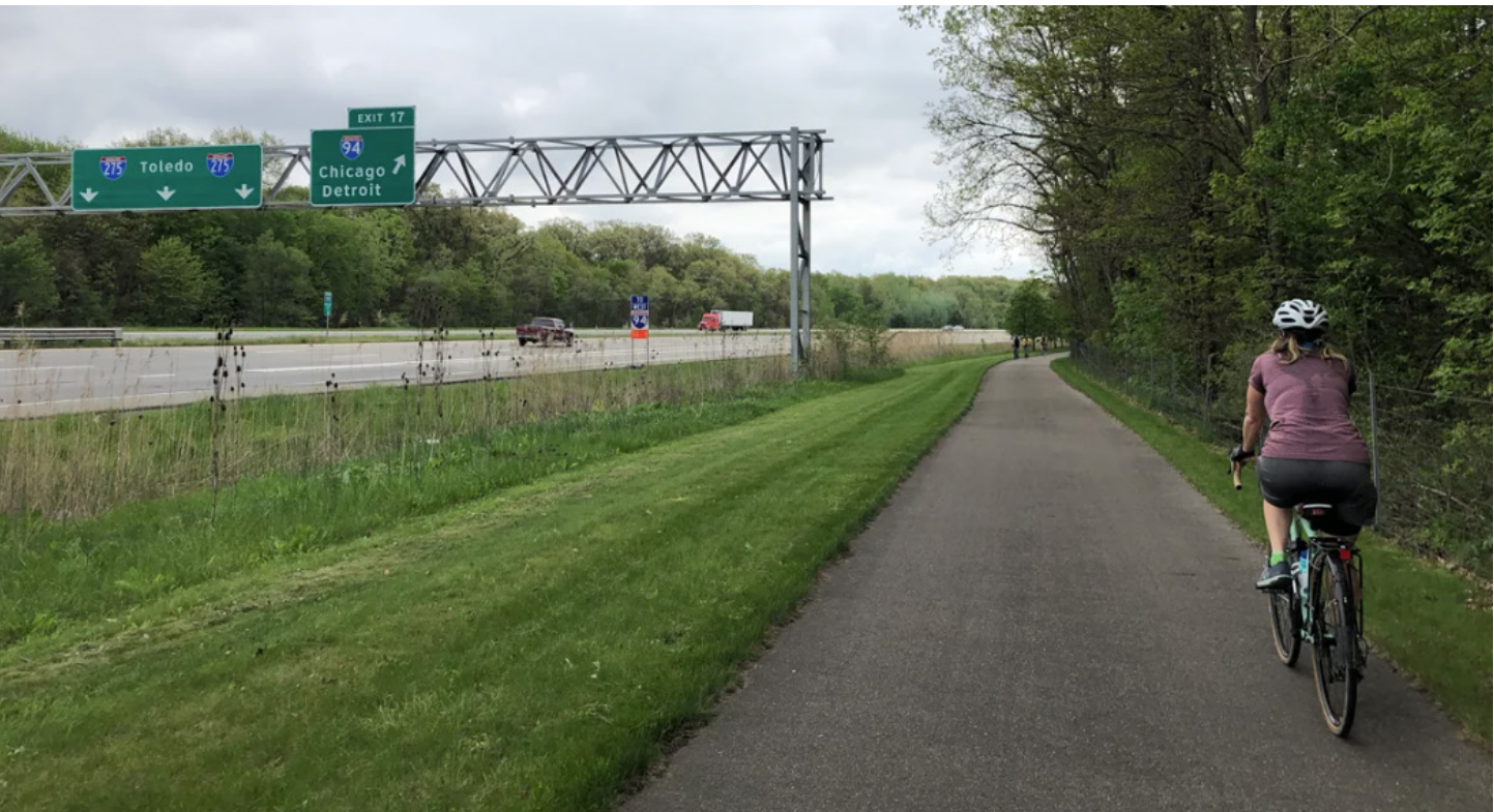
The I-275 Metro Trail features a wide asphalt path with ample buffer from the interstate, illustrating how separation and space can enhance comfort and usability along a highway corridor.
